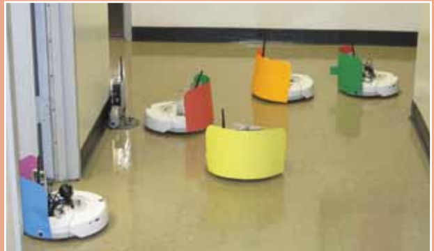
Figure A. Convoy of four robots following a leader. The red robot leaves the group to charge its battery at a base station.
